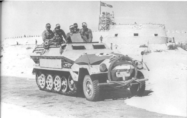
An Sd.Kfz.251/1 Ausf.B passes a captured fortification in Cyrenaica. A German national flag can be seen attached over the front of the vehicle for aerial recognition. The halftrack has received a full application of yellow-brown, which was the official camouflage colour scheme of the Afrika Korps.
