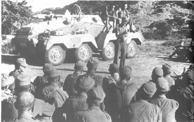
An officer instils courage and determination into his men during operations in Tunisia. The vehicle parked in the background is a 'Puma' Sd.Kfz.234/3 variant, mounting the 7.5cm KwK L/24 gun. This eight-wheeled vehicle was used mainly for reconnaissance duties.
