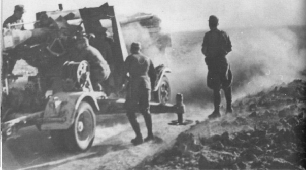
An 8.8cm flak gun being fired against a ground target from its limber. Out on the battlefield the 8.8cm proved a very versatile weapon and continued being used in a dual anti-tank and anti-aircraft role throughout the campaign in North Africa.
